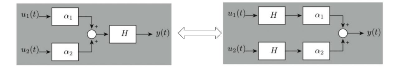
The linearity exists in both time domain and frequency domain
