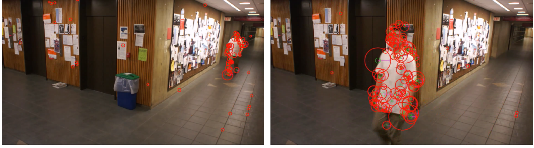
Figure 1: Two key frames of two videos with same event. The red points are extracted MOSIFT [6] features whose scale of motion are indicated by the size of circles.
