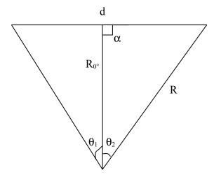
Diagram 3: trigonometric calculation for 90° heading;  $\theta_1 \le 0^\circ$ ,  $\theta_2 \ge 0^\circ$ ,  $R_0 = 17.75$ cm,  $\alpha = 90^\circ$
