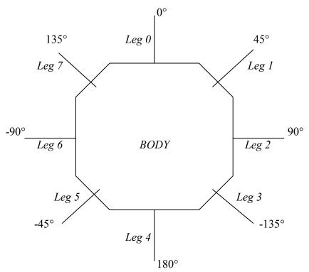
Diagram 1: leg headings for forward motion
