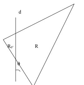
Diagram 4: trigonometric calculation for 45° heading;  $R_0$ °=17.75cm,  $\alpha$ =45°
