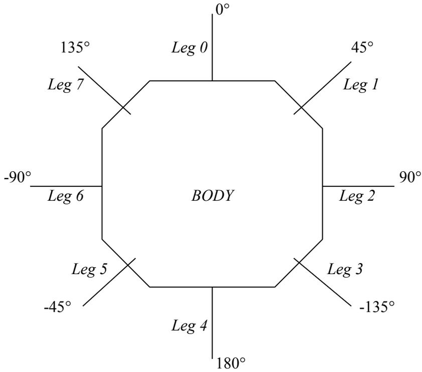
Diagram 1: leg headings for forward motion
