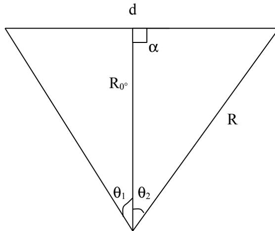
Diagram 3: trigonometric calculation for  $90^\circ$  heading;  $\theta_1 \leq 0^\circ$ ,  $\theta_2 \geq 0^\circ$ ,  $R_0 = 17.75\text{cm}$ ,  $\alpha = 90^\circ$
