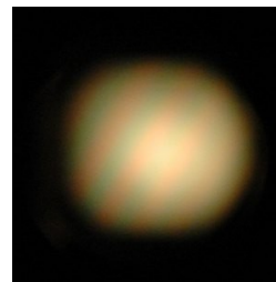
Figure 5.3: Faint red and green fringes farther from zero path difference
