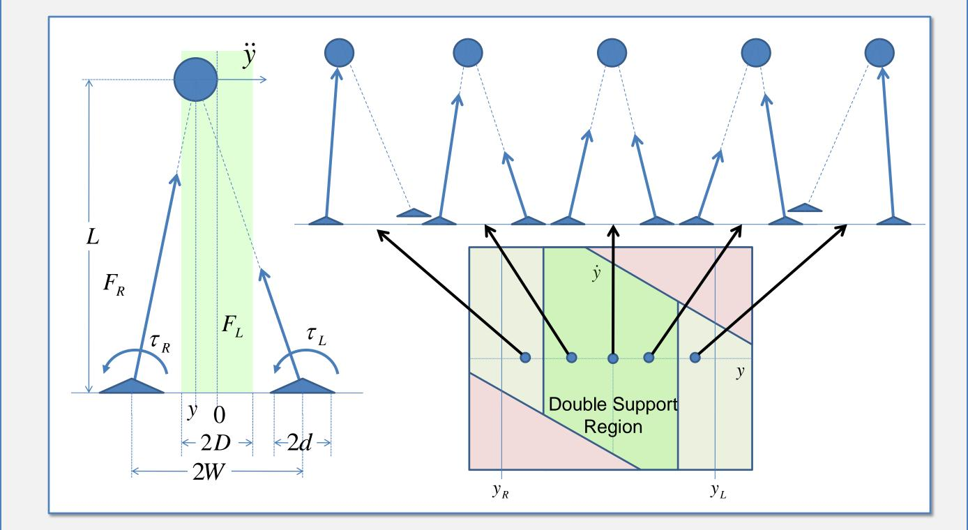
We define the weights using the position of the center of mass. While in a "double support region," the weights vary linearly. In single support, one weight is zero and the other is one.
