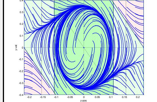
A controller can be derived to drive the energy error asymptotically to zero. We can then use the inverse dynamics of the linear biped model to generate nonlinear ankle torque policies for any desired energy.
