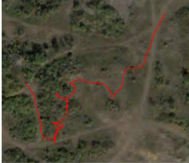
Figure 2: UGVs navigating with a limited perception range will often execute highly suboptimal paths. The path above was executed by a large UGV whose goal was to navigate to the goal at the left portion of the environment using an onboard perception system with a range of approximately 15 meters. Due to its limited visibility range, the UGV lost significant time navigating through the heavy vegetation, even requiring a human intervention at one point.
