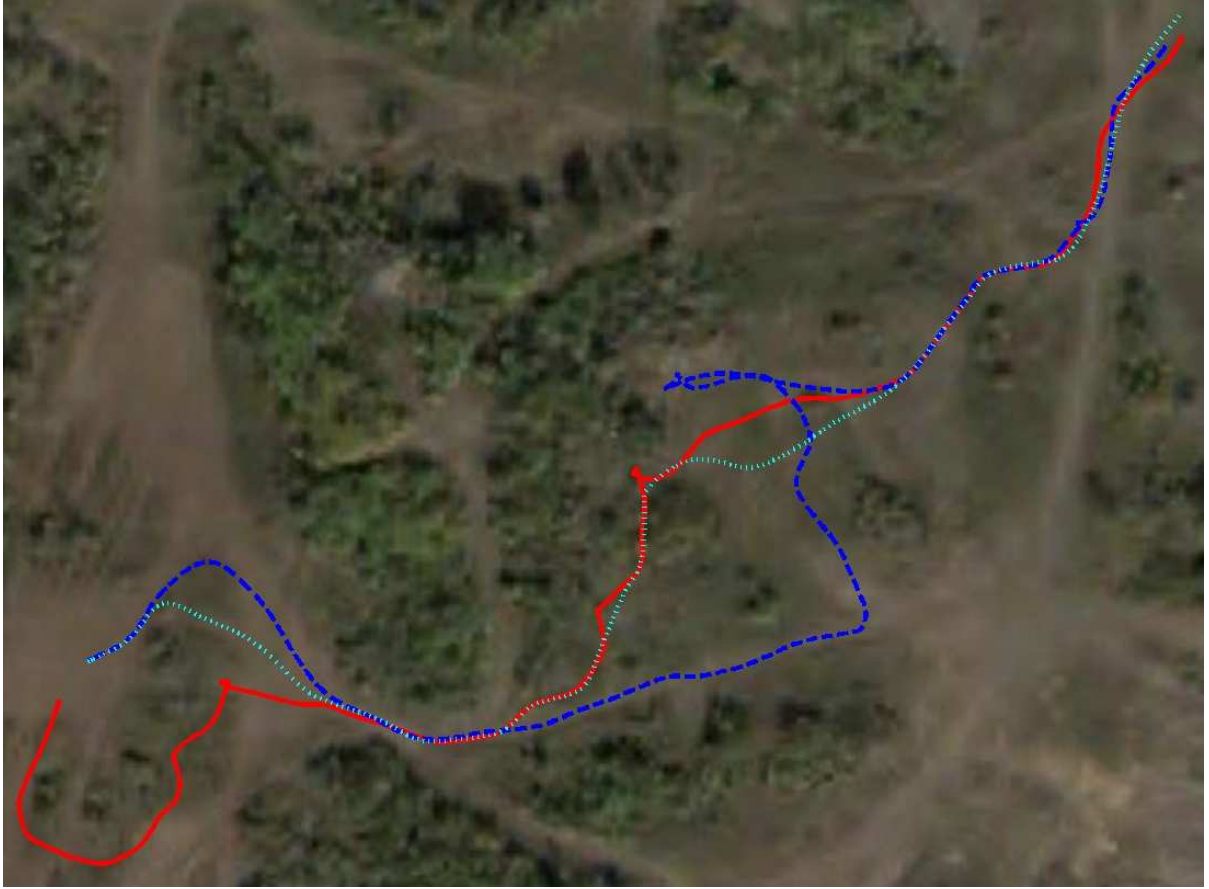
Figure 18: Comparison of paths executed by our robot for shown course when using only on-board perception (in solid red), and with MOLL (in dashed blue) and FROLL (in dotted cyan) used in real-time on-board the robot. Course started at the top right and ended at the bottom left.
