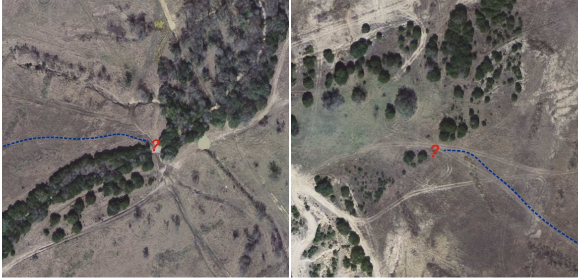
Figure 36: We plan to develop an uncertainty resolution technique that can distinguish between situations such as those above. In the left image, resolving the uncertainty at this pinch point through a human query can potentially save significant time and travel distance. In the right image, the outcome of a human query cannot significantly effect the path.
