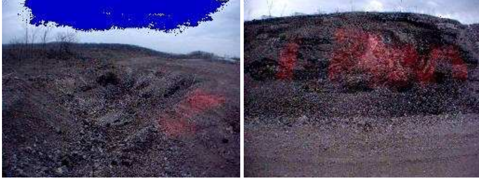
Figure 33: Additional examples of novel instances identified during later traversal (red shade): first encounter with a ditch (left) and a large, heavily-sloped pile of rocks (right).
