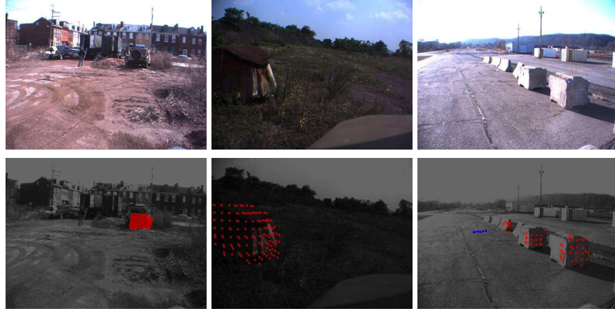
Figure 26: Sample hand labeled examples in the 'other man-made' class used for validation of dimensionality reduction effectiveness. This category excluded instances of barrels which were used as a separate class.
