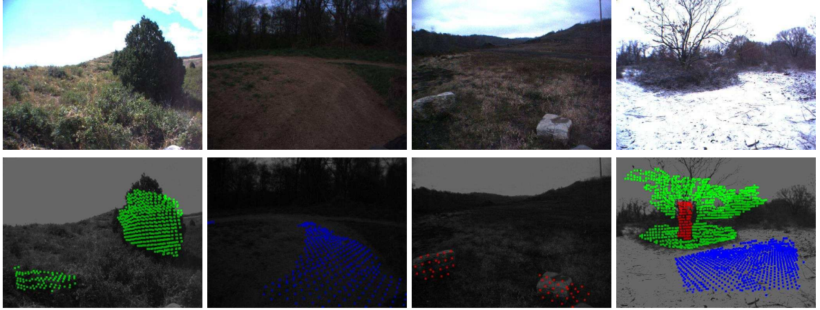
Figure 25: Examples of hand labeled class categories (bush, road / grass, rocks, tree trunk, tree branches, etc.)
