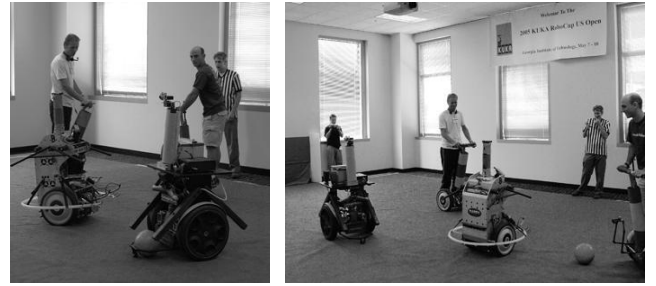
Figure 5: The left figure shows our Segway robot holding the ball and turning to search for its teammate. The right figure shows our Segway robot positioning to receive a pass, and being marked by the NSI robot.
