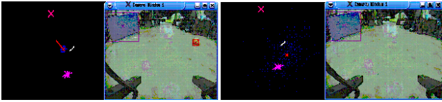
Figure 4: In both figures, the red and pink cross represent the two goals, and each blue dot represents the one of the particle estimation of the ball position. In the left figure, the ball is visible to the robot. In the right figure, the ball is out of sight and the particles are scattered
