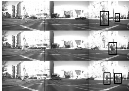
Figure 6.19. Visual images from the tri-camera system. Block boxes indicate the detected and tracked pedestrians.
