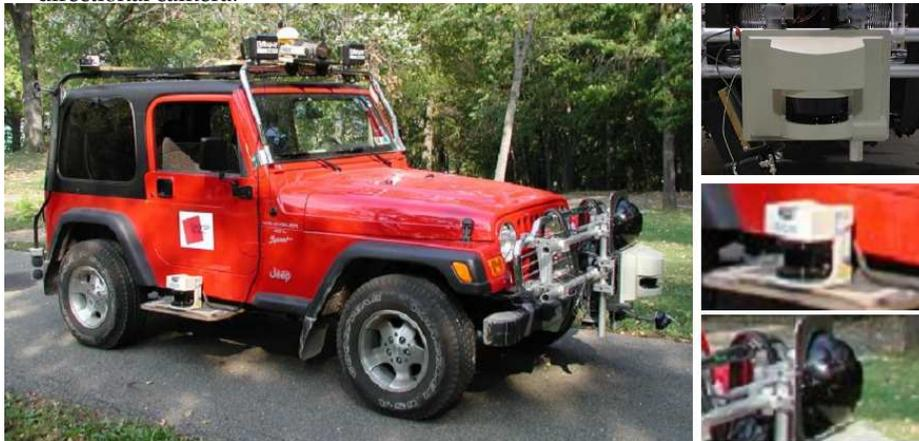
Figure 1.8. Right: the Navlab11 testbed. Left: SICK LMS221, SICK LMS291 and the tri-camera system.
