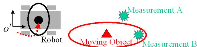
Figure 6.2. Performing detection, data association and motion modelling with respect to a temporary global coordinate system.
