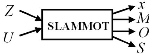
(c) the simultaneous localization, mapping and moving object tracking (SLAMMOT) process
