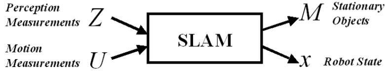
(a) the simultaneous localization and mapping (SLAM) process
