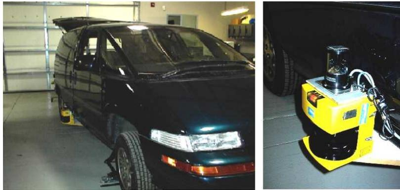
Figure 1.7. Left: the Navlab8 testbed. Right: the SICK PLS100 and the omni-directional camera.
