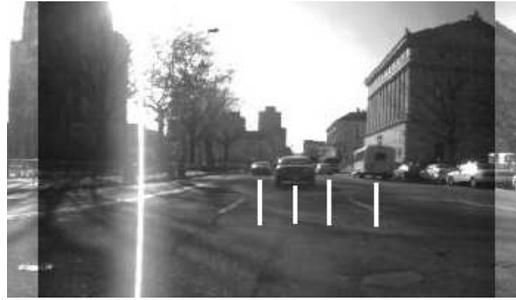
Figure 6.14. The partial image from the tri-camera system. Four lines indicate the detected vehicles.
