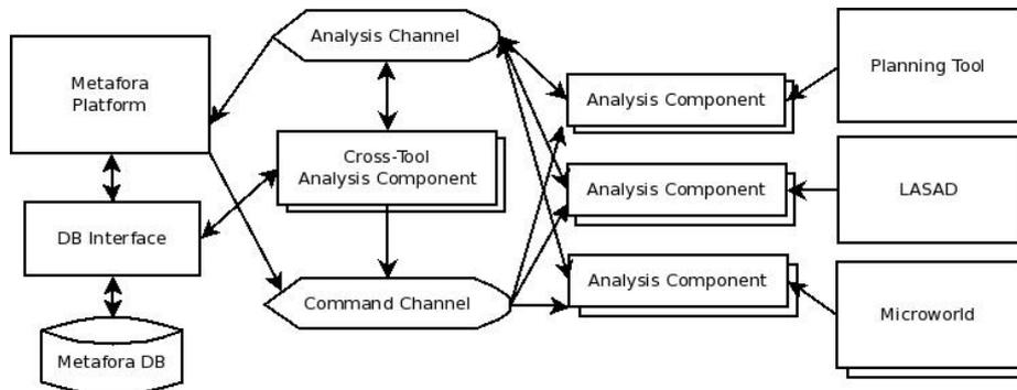
**Fig. 4.** The communication structure between tools in the Metafora system.
