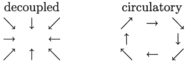
Fig. 9. A decoupled field (left) with symmetric \mathbf{k}_s and a circulatory field (right) with skew-symmetric \mathbf{k}_s .
