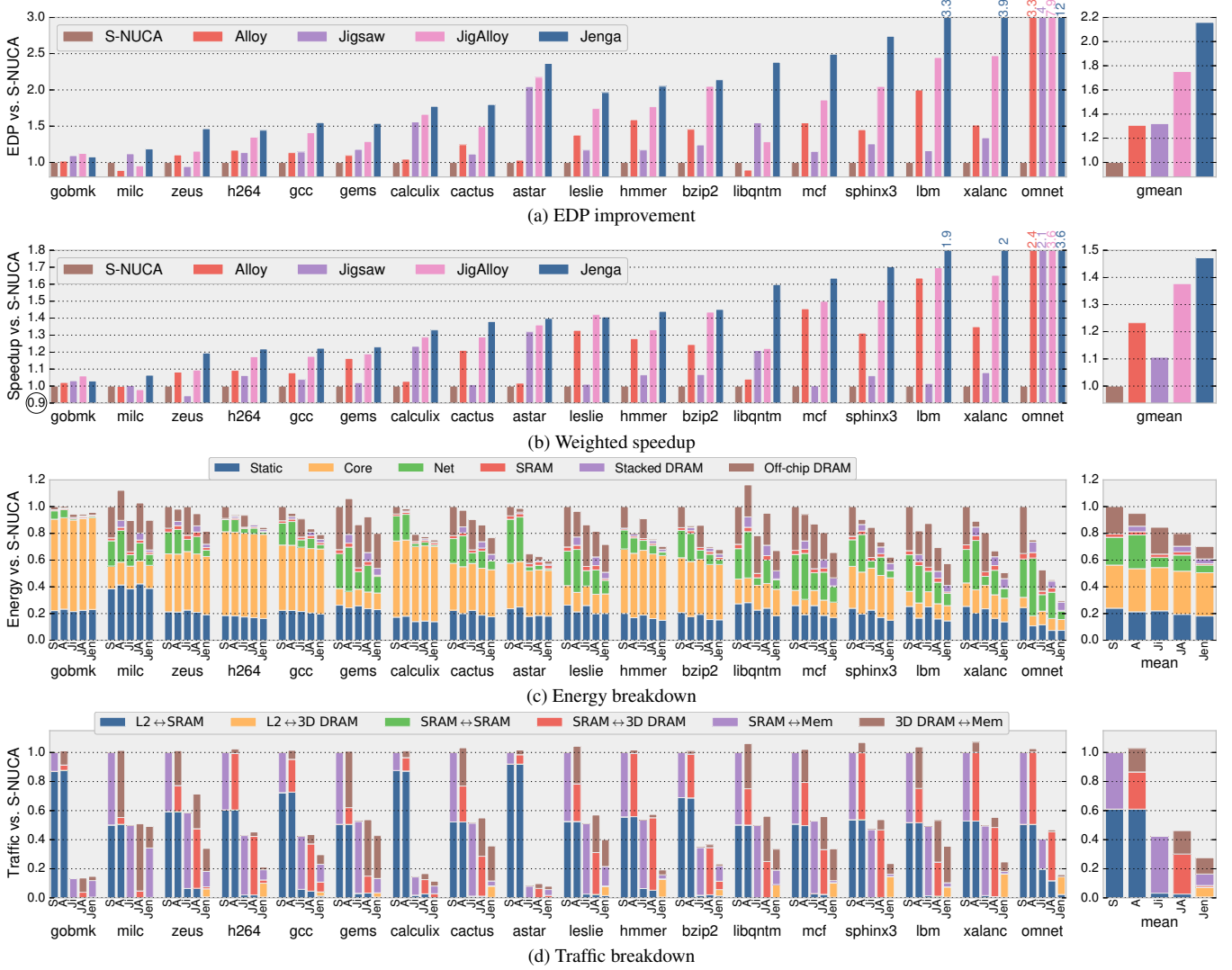
Figure 19: Simulation results on 36 concurrent copies SPEC CPU2006 apps (rate mode).
