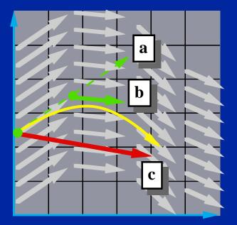
a. Compute an Euler step  $\Delta \mathbf{x} = \Delta t \mathbf{f}(\mathbf{x},t)$ b. Evaluate f at the midpoint  $\mathbf{f}_{mid} = \mathbf{f}\left(\frac{\mathbf{x} + \Delta \mathbf{x}}{2}, \frac{t + \Delta t}{2}\right)$ c. Take a step using the midpoint value  $\mathbf{x}(t + \Delta t) = \mathbf{x}(t) + \Delta t \mathbf{f}_{mid}$
