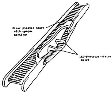
Figure 3: Cutaway view of an Allison Research Slider
