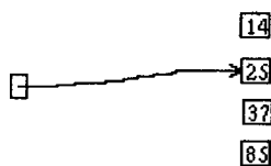
Figure 1. Pictorial representation of a POINTER TO INTEGER 2 .
