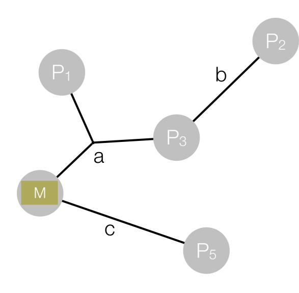
Program: network of processes connected by channels
