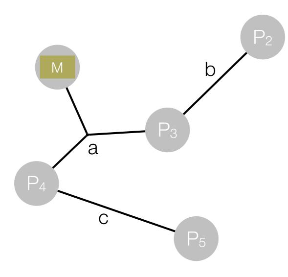
Program: network of processes connected by channels
