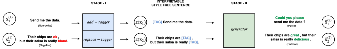
Figure 3: Our proposed approach: tag and generate . The tagger infers the interpretable style free sentence z(\mathbf{x}_i) for an input \mathbf{x}_i^{(1)} in source style \mathcal{S}_1 . The generator transforms \mathbf{x}_i^{(1)} into \hat{\mathbf{x}}_i^{(2)} which is in target style \mathcal{S}_2 .
