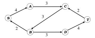
Figure 16.3: Residual graph resulting from pushing 2 units of flow along the path s-b-c-t in the graph in Figure 16.1.
