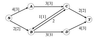
Figure 16.2: A network flow graph with positive flow shown using "capacity[flow]" notation.
