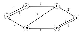
Figure 16.4: Residual graph resulting from pushing 3 units of flow along the path s-a-c-b-d-t in the graph in Figure 16.3.
