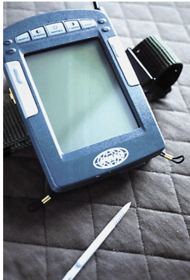
Figure 4: TIA-P Wearable Computer
