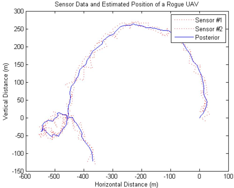
Figure 3: The UAV's predicted path (blue) from  $t = 0$  to  $t = 100$ . Observations from both towers are shown in red.
