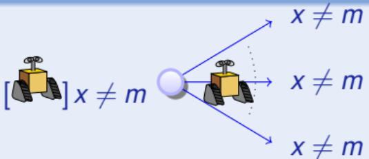
$$\underbrace{x \neq m \wedge b > 0}_{\text{init}} \rightarrow \left[ \underbrace{\left( (\text{if}(SB(x, m)) \quad a := -b) ; \ x' = v, v' = a \right)^*}_{\text{all runs}} \right] \underbrace{x \neq m}_{\text{post}}$$
