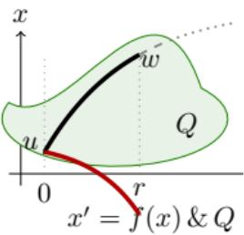
DI  $[x' = f(x)]e \geq 0 \leftarrow e \geq 0 \wedge [x' = f(x)](e)' \geq 0$
