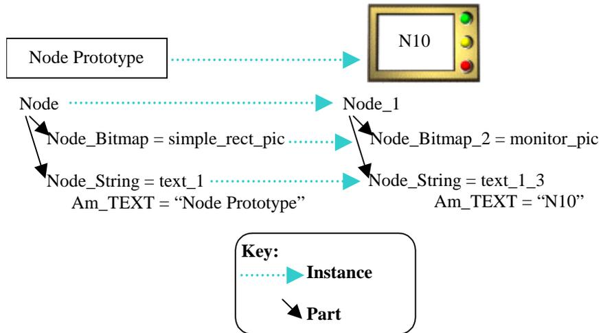
**Figure 2:** When an instance is made of the node prototype, an instance is also made of each of the parts.
