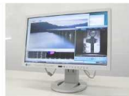
The 20-inch model "FlexScan EV2023W-H" adopts the "FlexStand" mechanism with a 225mm height adjustment range.
