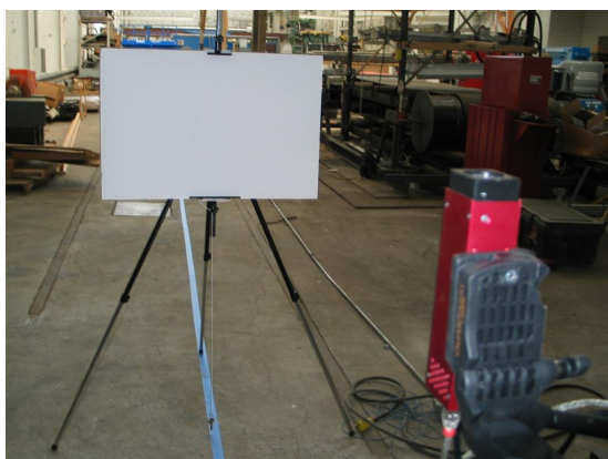
Figure 3: Experimental setup for characterizing the effects of range, reflectance, and angle of incidence have on range measurements of a flash lidar device.
