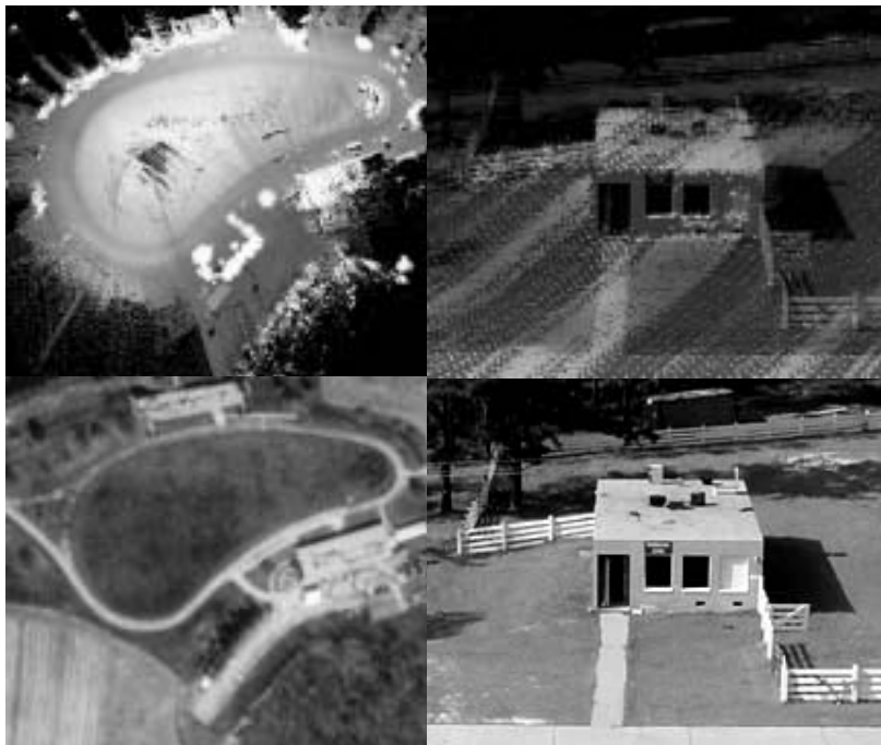
Fig. 13. UAV Mapping Performance At Global and Local Scales. (Top Left) Digital Elevation Map produced by the UAV. (Bottom Left) Orthophoto from another source. (Top Right) Fused lidar and color data of a building. (Bottom right) Photograph from same perspective.
