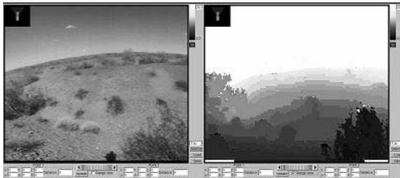
Fig. 6. Computational Image Plane Registration. Dense range data is relatively easy to correspond with appearance data given calibrated inter-sensor poses and the ability to correctly associate historical vehicle poses with range pixels.
