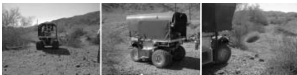
Fig. 19. Photos of the UGV at the top of a lethal ledge, attempting to enter the gully. Even with three photos, the ledge is not easily observed. The operators, with less information than is shown in this figure, chose to move forward, leading to an ESTOP during teleoperation.
