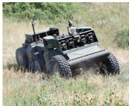
(a) Crusher, a six-wheeled skid-steered mobile robot
