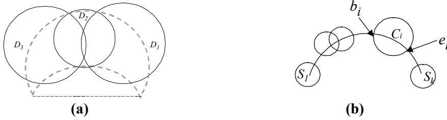
Fig 8: (a) If k = 2 , our reduced test will only test pairs (D_1, D_2) and (D_2, D_3) . The resulting interval, H , is shown by two arcs. Not all arcs in interval H will intersect disks D_1 and D_3 in order. (b) Checking the order requirement for an arc A^*
