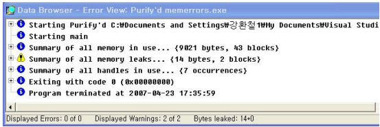
A2-2 Detection Defect with Visual Studio 2005 C-Compiler
