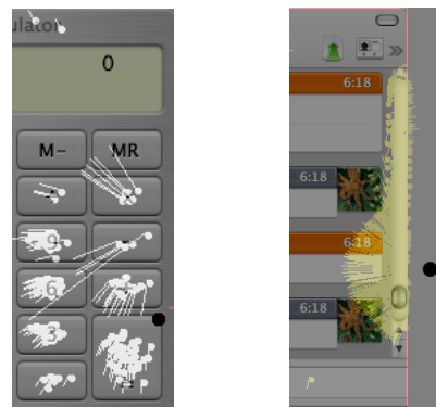
Figure 1: (left) An illustration of how clicks (white dots) collect on commonly used buttons in a calculator, creating a cumulative force (white lines) on the pointer (black dot). (right) The cumulative force (yellow lines) on the dragged pointer as it leaves the bounds of a scrollbar in an IM client.
