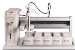
The Versatile Automated Sampler Transport (VAST) rapidly injects samples into the NMR spectroscope.
