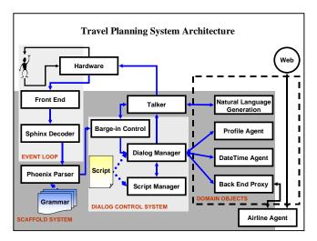
Figure 1: The system architecture
