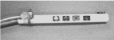
Figure 3. The stick with attached tracker. Note the location of the thumb button on the dorsal face of the stick.
