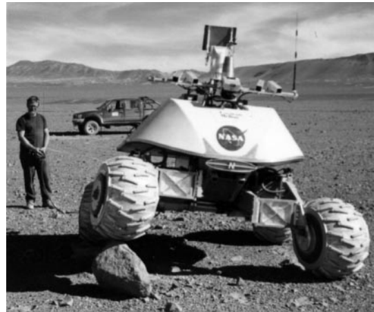
Figure 4: Nomad perches on a rock, demonstrating the averaging suspension and the stability-enhancing large footprint
