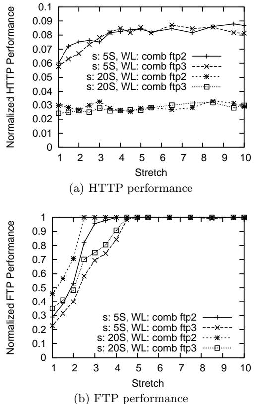
**Figure 6: Performance of HTTP and FTP flows with optimal static assignment of APs to the three non-overlapping channels. The transmit power level is set at 15dBm, corresponding to a reception range of 31m.**
