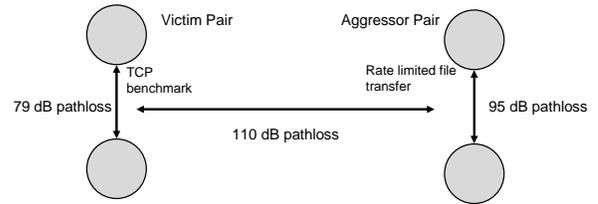
Figure 11: Laboratory Interference Test Topology
