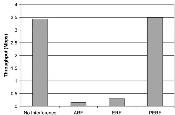
Figure 13: Lab Interference Test - Unlimited Rate
