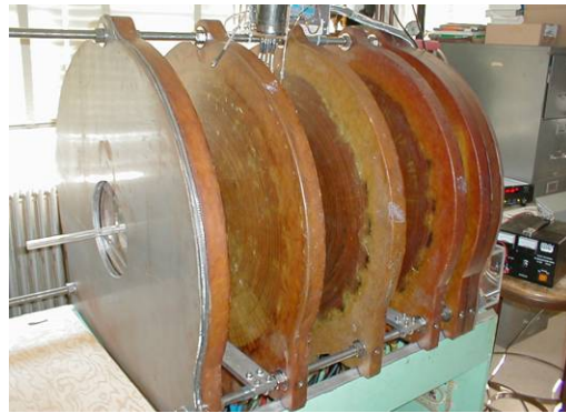
FIG. 2.6 Solenoid magnet focusing for the electron beam. The XWING is placed at the centre of the solenoids.
