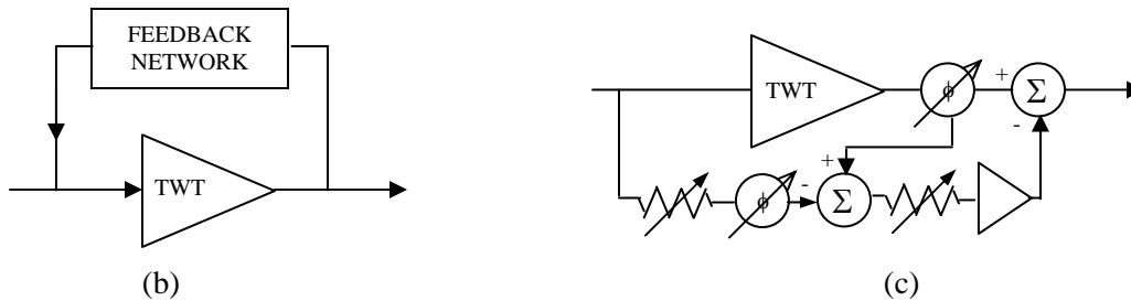
FIG. 1.5 Prevalent linearization schemes: (a) Predistortion (b) Feedback and (c) Feedforward linearization.
