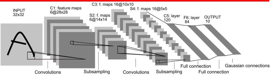
C1: Convolutional layer with 6 feature maps of size 28x28. C1<sub>k</sub> (k=1...6)
