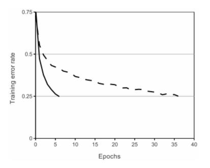
A four-layer convolutional neural network with ReLUs (solid line) reaches a 25% training error rate on CIFAR-10 six times faster than an equivalent network with tanh neurons
