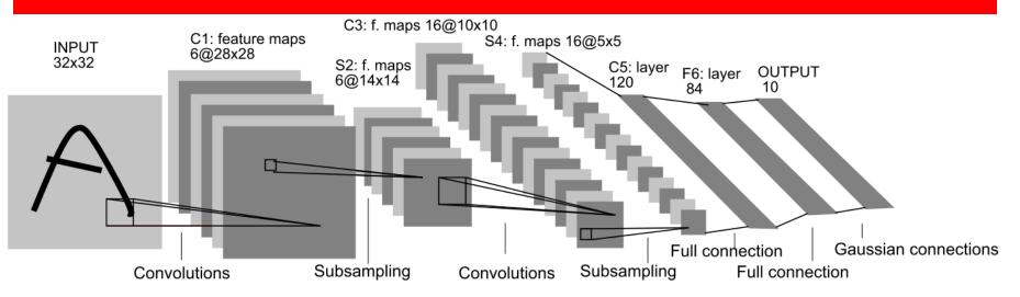
Layer F6: 84 fully connected units. 84\*(120+1)=10164 trainable parameters and connections.
