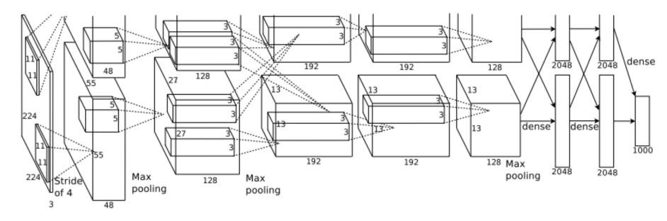
**The first convolutional layer** filters the  $224 \times 224 \times 3$  input image with 96 kernels of size  $11 \times 11 \times 3$  with a stride of 4 pixels (this is the distance between the receptive field centers of neighboring neurons in the kernel map. 224/4=56
