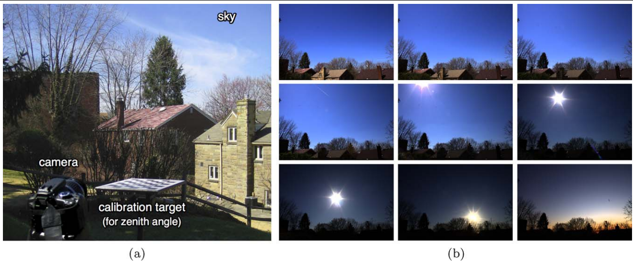
Fig. 4 Ground truth data acquisition. a Acquisition setup. The calibration target, placed on a tripod in front of the camera and levelled with the ground, is used to recover the camera zenith angle. b Exam-
