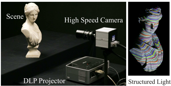
Fig. 2 Illumination and acquisition setup for structured light based 3D reconstruction: (a) The Photron high speed camera is placed vertically above the Infocus DLP projector in our acquisition setup. A vertical plane is placed at known distance behind the scene to enable finding correspondences. (b) The scene (statue) is illuminated using only a single pattern, as shown on the right. This pattern is static when viewed directly by unaided eyes. At high-frame rate, however, it is decomposed into a high-frequency patterns by the DLP projector.
