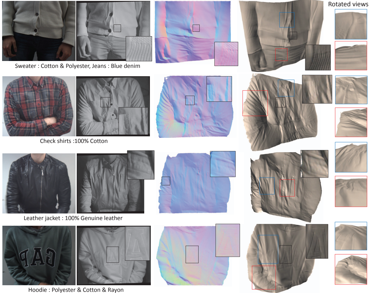
Figure 10. Results of our shape estimation using various real-world clothings - Sweater, Check shirts, Leather Jacket, and Hoodie. From the left, each column presents visible images, NIR images, Normal map and Reconstructed 3D mesh. Note that our method requires only a NIR image for the input, the visible images are provided for visual comparison of reflectance.
