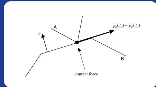
$(\dot{p}_a(t_0) - \dot{p}_b(t_0)) \cdot n = 0$ Resting contact.
