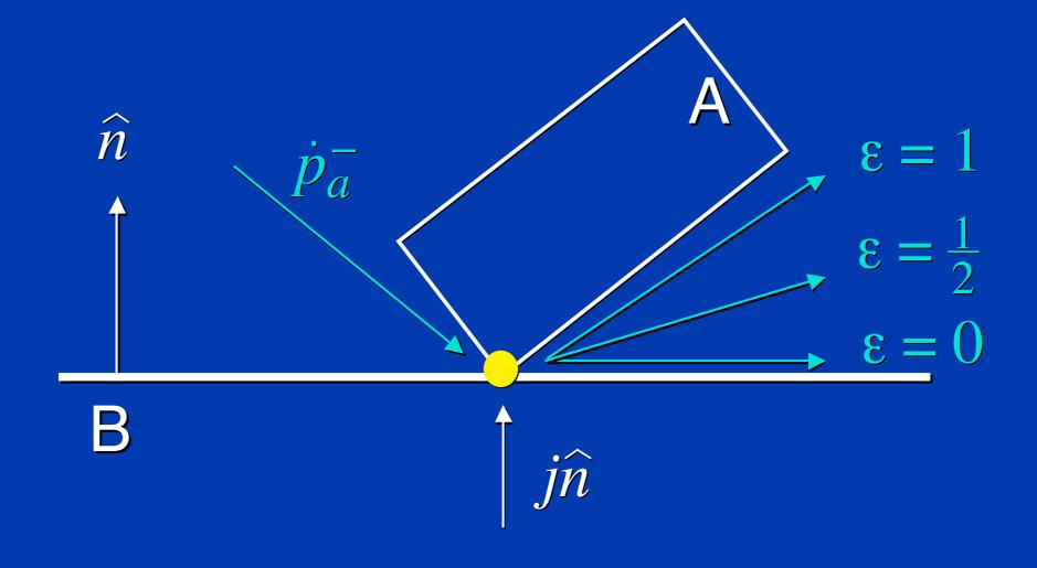
$$v_{a}^{+}(t_{0}) = v_{a}^{-}(t_{0}) + \frac{j\hat{n}(t_{0})}{M_{a}}$$
