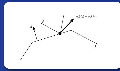
$(\dot{p}_a(t_0) - \dot{p}_b(t_0)) \cdot n > 0$ No collision.
