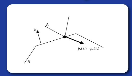
$(\dot{p}_a(t_0) - \dot{p}_b(t_0)) \cdot n < 0$ Impulse collision.
