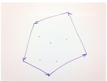
This figure shows the convex hull of 10 points.
