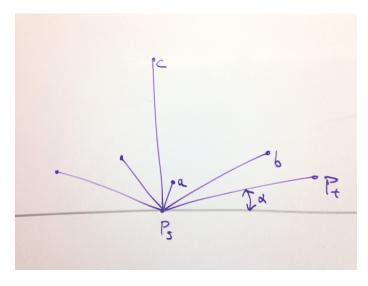
All the other points must be to the left of segment  $(P_s, P_t)$ . We can continue this process to find the point  $P_u$  which is the one with the smallest angle with respect to  $(P_s, P_t)$ . This process is continued until all the points are exhausted. The running time is O(n) to find each segment. There are O(n) segments, so the algorithm is  $O(n^2)$ .
