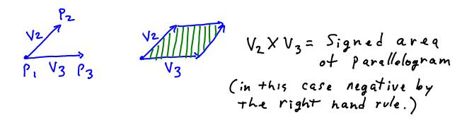
Here is an implementation of this test in ocaml which returns 1 if  $p_3$  is LEFT of ray  $p_1 \to p_2$ , -1 if RIGHT, and 0 if ON.
