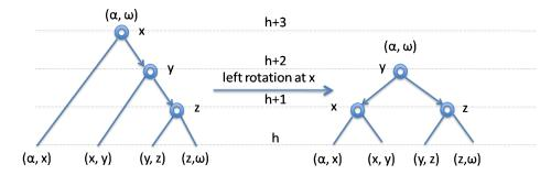
We fix this with a left rotation at x, the result of which is displayed to the right. Because the height of the overall tree is reduced to its original h+2, no further rotation higher up in the tree will be necessary.
