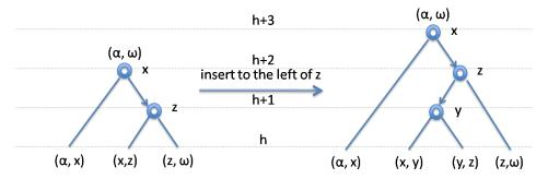
In the situation on the right, the subtrees labeled  $(\alpha,x)$  and  $(z,\omega)$  must have exactly height h, but only one of (x,y) and (y,z) does. In this case, a single left rotation alone will not restore the invariant (see Exercise 1). Instead, we apply a so-called *double rotation*: first a *right* rotation at z, then a *left* rotation at the root labeled x. When we do this we obtain the picture on the right, restoring the height invariant.
