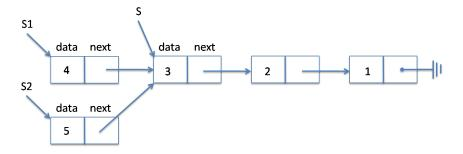
All three stacks share nodes 3, 2 and 1. Observe furthermore that the second call to push operated on S, which remained unchanged after the first call. At this point, a pop on S would result in a fourth stack, say S3, which points to node 2.
