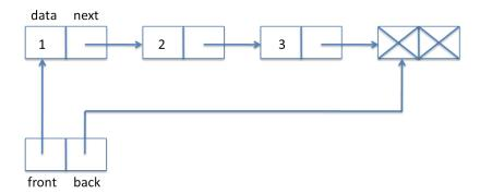
A queue is implemented as a struct with a front and back field. The front field points to the front of the queue, the back field points to the back of the queue. We need these two pointers so we can efficiently access both ends of the queue, which is necessary since dequeue (front) and enqueue (back) access different ends of the list.
