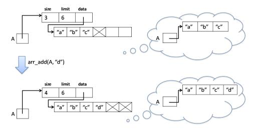
The images to the left above represent how the data structure is actually stored in memory, and the images in the thought bubbles to the right represent how the client of our array library can think about the data structure after an arr\_add operation.
