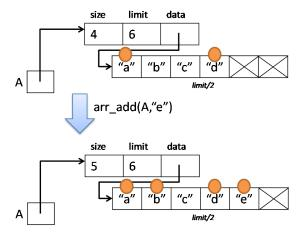
In the cases where the addition does completely fill the array, we need to copy over every element in the old array into a new, larger array in order to preserve the A->size < A->limit data structure invariant. This
