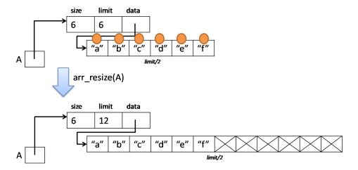
After the resize, exactly half the array is full, so our data structure invariant for tokens doesn't require us to have any tokens in reserve. This means that the data structure invariant is preserved in this case as well. In general, the number of tokens associated with an unbounded array is 2size - limit.
