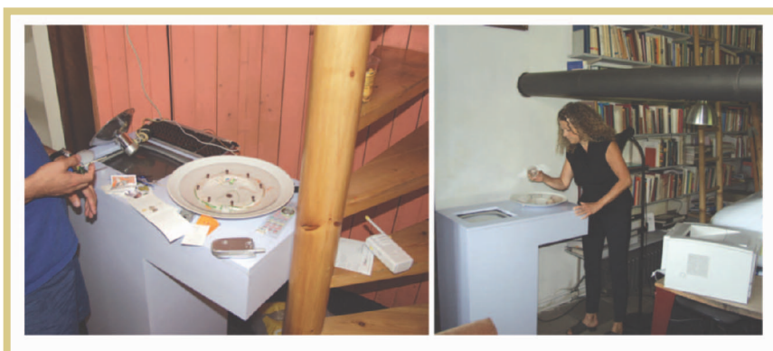
Figure 7. A high-tech prototype's technical construction. (a) The bowl is connected with a spring to an electromotor, (b) a camera with fisheye lens is positioned pointing upwards below the bowl, and (c) a PC connects all elements.
