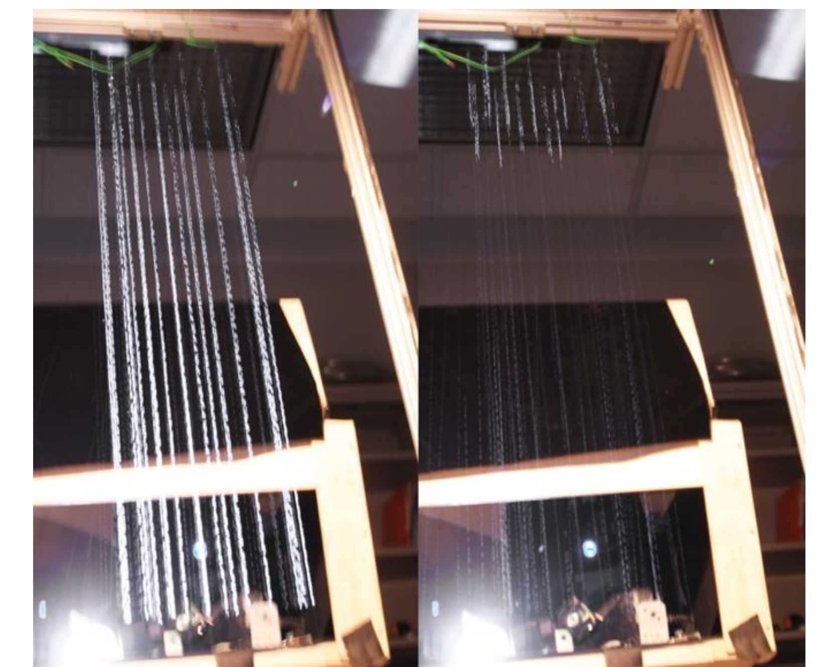
Fig. 8: Results for system at 120 Hz against cluttered background. Left/right shows full/adaptive illumination.
