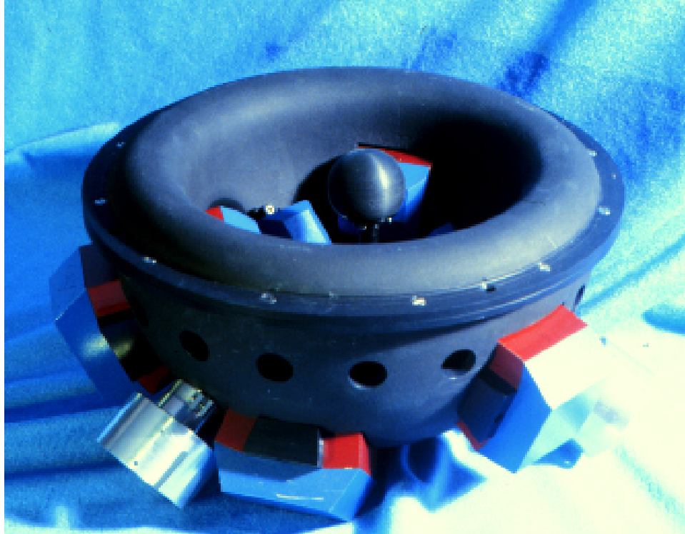
Figure 6.2: New Fabricated Lorentz Levitation Haptic Device
