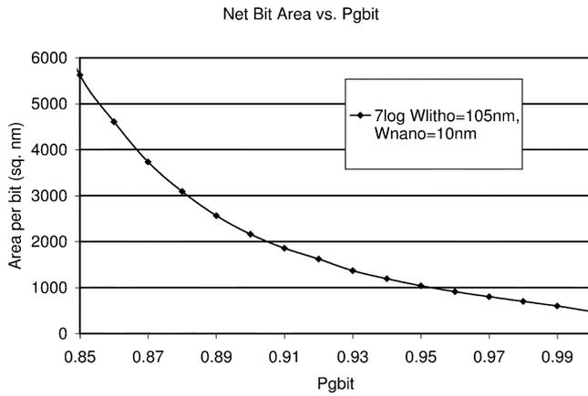
Fig. 13. Net memory bit density as a function of  $P_{\text{gbit}}$  (7 log,  $W_{\text{litho}} = 105$ ,  $W_{\text{nano}} = 10$ ,  $P_c = 0.95$ ,  $P_{\text{junc}} = 0.9999$ ,  $P_{\text{bank-yield}} = 0.98$ ).
