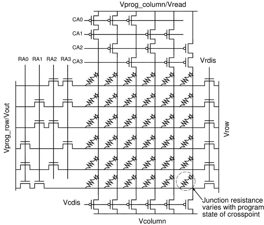
Fig. 3. Rough circuit equivalent for nanoscale memory.
