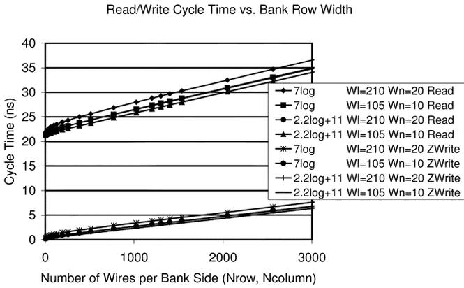
Fig. 7. Precharge read and zero write cycle time as a function of  $N_{\text{row}}$  with  $R_{\text{contact}} = 1 \text{ M}\Omega$  and  $R_{\text{onodiode}} = 0.1 \text{ M}\Omega$ .
