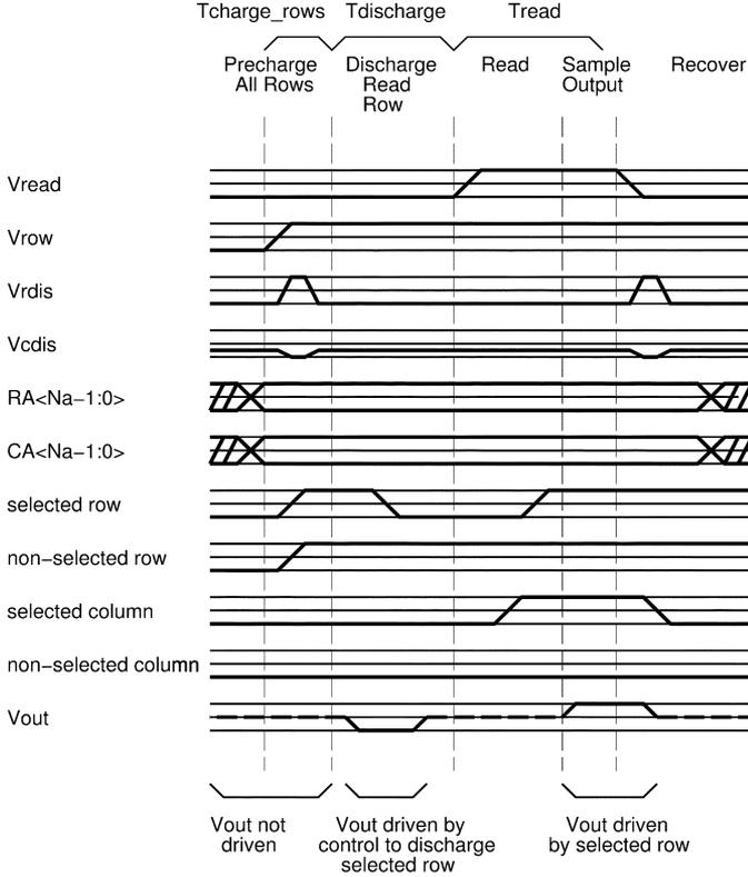
Fig. 4. Precharge read timing diagram. Diagram shows a read of an “on” junction.
