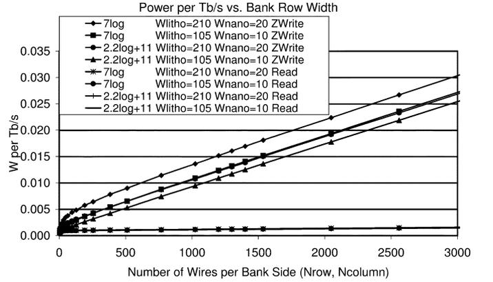
Fig. 9. Power per Tb/s a function of  $N_{\text{row}}$  for precharge read and zero write.
