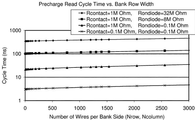
Fig. 8. Precharge read cycle time as a function of  $N_{\text{row}}$  for various resistances.  $W_{\text{liitho}} = 105 \text{ nm}$ ,  $W_{\text{nano}} = 10 \text{ nm}$ ,  $7 \lceil \log_2(N) \rceil$  addressing.
