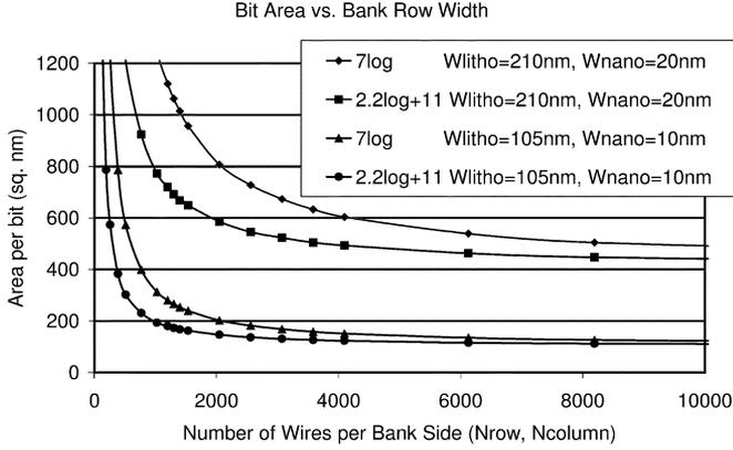
Fig. 5. Raw memory bit density as a function of  $N_{\text{row}}$ .
