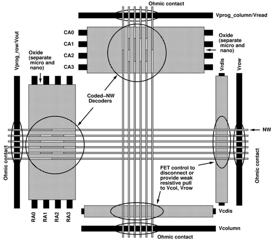
Fig. 2. Nanoscale memory array bank; for clarity, only a small ( $6 \times 6$ ) NW crossbar is shown. A typical array might have 100–3000 nanoscale wires on each side and be addressed by 35–60 microscale wires.
