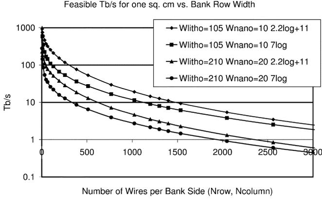
Fig. 11. Feasible read bandwidth for one  $\text{cm}^2$  as a function of  $N_{\text{row}}$ .
