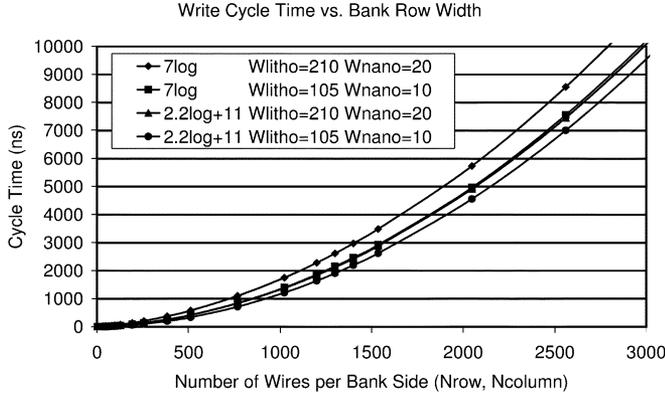
Fig. 6. Random write cycle time as a function of  $N_{\text{row}}$  with  $R_{\text{contact}} = 1 \text{ M}\Omega$  and  $R_{\text{onodiode}} = 0.1 \text{ M}\Omega$ .
