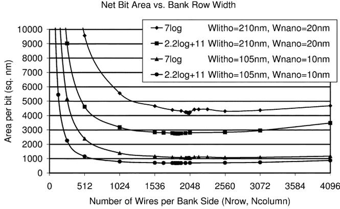
Fig. 12. Net memory bit density as a function of  $N_{\text{row}}$  ( $P_c = 0.95$ ,  $P_{\text{junc}} = 0.9999$ ,  $P_{\text{gbit}} = 0.95$ ,  $P_{\text{bank-yield}} = 0.98$ ).
