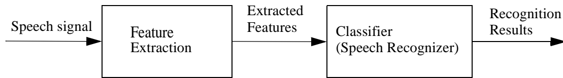
Figure 2.1. Block diagram of two-stage processing in speech recognition. The first stage is feature extraction, and the second stage is classification.
