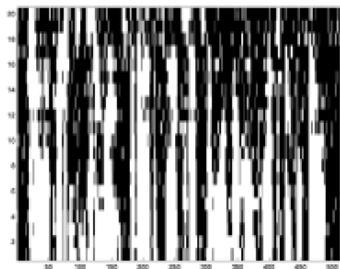
Figure 6.8 Estimated mask for an utterance corrupted with white noise to 10dB. The horizontal axis is frame number and the vertical axis is Mel filter number. The black pixels indicate corrupt or “missing” features. The white pixels indicate reliable features.
